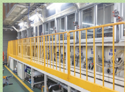
Cationic electrodeposition coating equipment at Nishi Ogaki Plant
