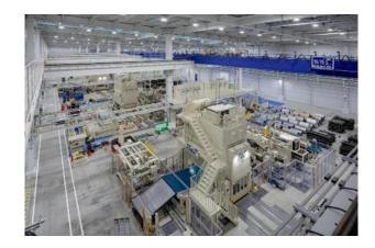
Mass production of stamping products such as ultra high strength parts and HEV battery cases
