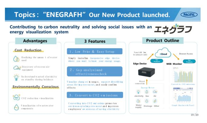
We have developed and launched ENEGRAPH in May, an edge device that collects usage data from meters and a web system. It collects usage data from production facilities that use electricity, gas, air, and water, and visualize them in real time through the cloud.
