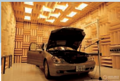
Soundproofing and vibration-proofing evaluation equipment
