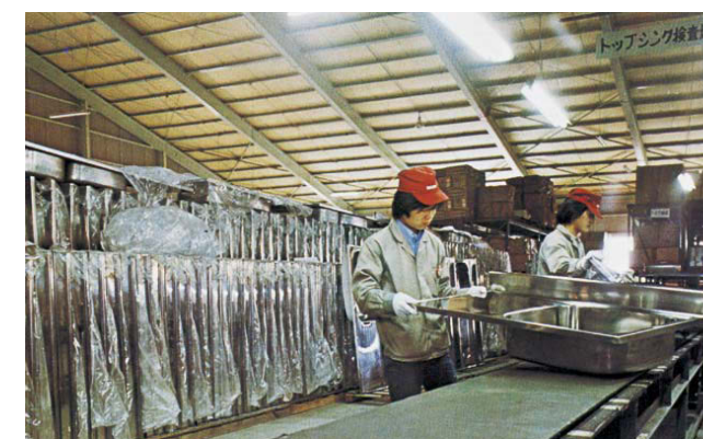
Kitchen sinks which were produced at the rate of 40 thousand units per year at one time at the Anjo factory by the housing equipment division from 1971.
