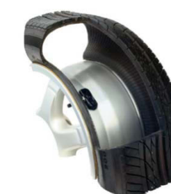
A TPMS transmitter mounted inside a tire.
