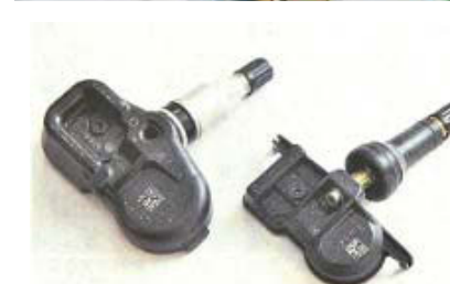
TPMS transmitters developed domestically for the first time in Japan, now mass-produced ever since.
